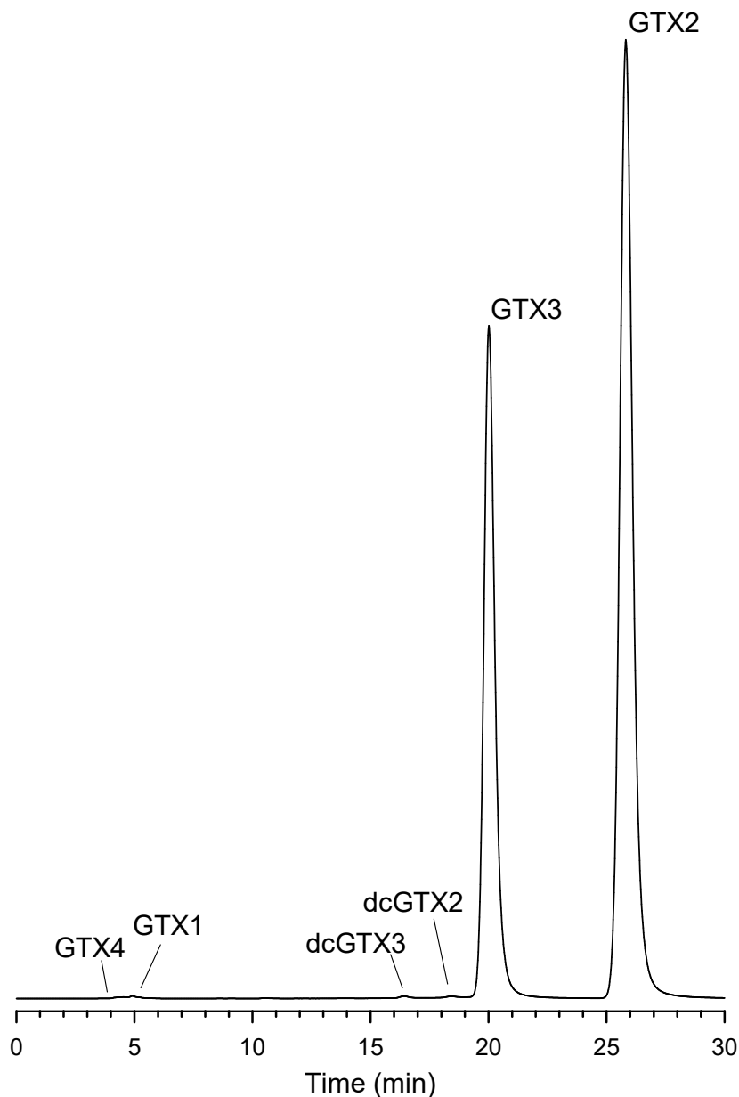
Figure 1: LC-ox-FLD analysis of CRM-GTX2&3-d. Retention times of related toxins are indicated. Conditions: Zorbax Bonus-RP column (250 × 4.6 mm i.d., 5 μm) at +35 °C; 0.8 mL/min of 5.5 mM ammonium phosphate with 11 mM sodium heptane sulphonate, pH 7.1; 5 μL injection; post column oxidation using 0.4 mL/min 5 mM periodic acid in 100 mM sodium phosphate at pH 7.8; reaction coil at +80 °C; effluent acidified with 0.4 mL/min 0.75 M nitric acid; fluorescence detection with excitation at 330 nm and emission at 390 nm.
