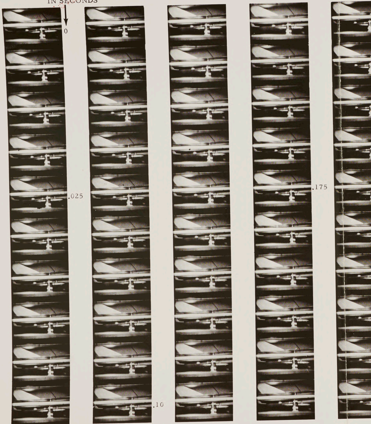
FIG. 5 (b) SIDE VIEW RUN NO. 12 - 40,000 FT., M = .85 , \alpha = 4.4^\circ TANK FULL, \psi = 0 FILM SPEED 750 FRAMES PER SECOND.
