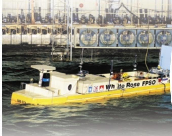
vessel for the White Rose Field. A series of model tests were conducted involving the producers, Oceanic Consulting, and NRC to measure mooring loads, green water and other factors affecting the FPSO in the field. NRC was the site for extensive testing of the Hibernia Gravity Base Structure that has operated successfully since 1996, the Terra Nova FPSO deployed in 2001, and the Cohasset-Panuke project.
