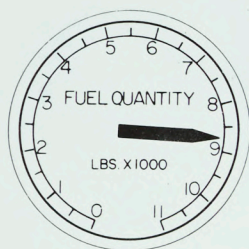
Figure 19. Fuel Quantity Meter
